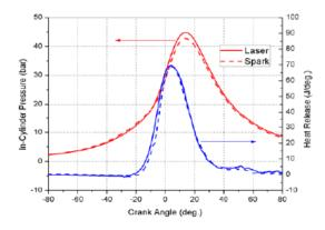
Fig.4.1 Comparison of in-cylinder pressure and heat release rate for LI and SI for wide open throttle (WOT) at 1500 rev/min, airfuel equivalence ratio  $\lambda \text{equ} = 1.2$
