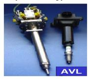
Fig. 3.3 Different laser sparkplugs developed worldwide
